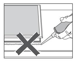
The sealing strip under the edge of the top part of the cooktop provides a sufficient seal for the worktop.
